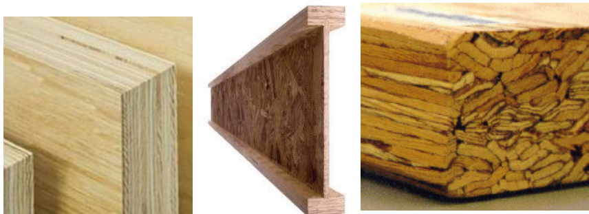
Figure 5 Laminated Veneer Lumber, Structural I-Joists, and Parallam
