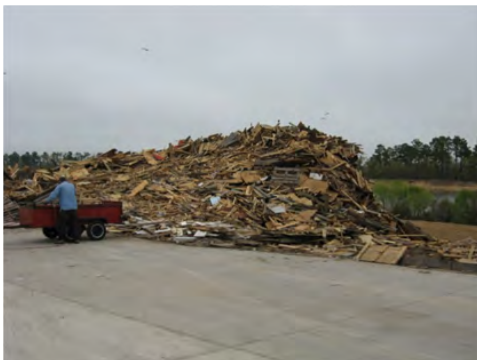
Lumber and pallets are stored on one corner of the New Hanover County landfill C&D pad until the material is scheduled for grinding.
