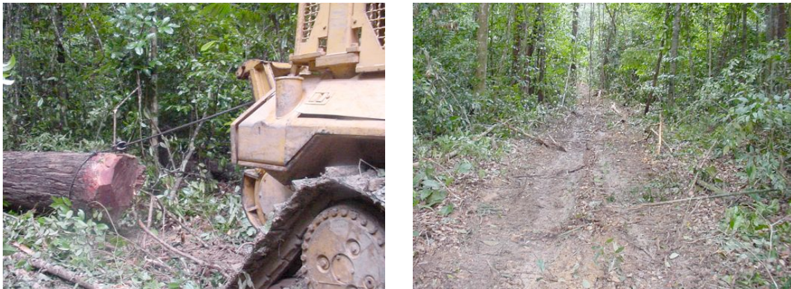
Figure 3a, 3b Skidding of logs in traditional logging often exposes considerable mineral soil
